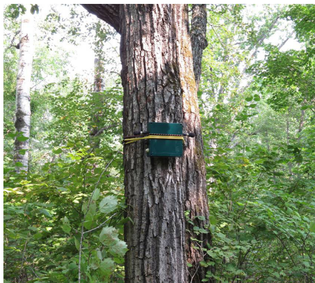
Fig. 1. The device (SongMeter SM2+), mounted on a tree at the State Nature Reserve «Bolshekhkhtsirsky» for the automated acoustic recording of male Far-East wapiti rutting calls.
